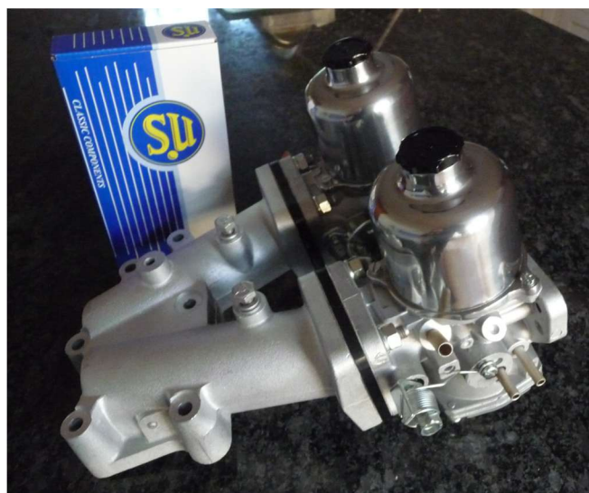
Richard's refurbished SU Carbs, prior to refitting
