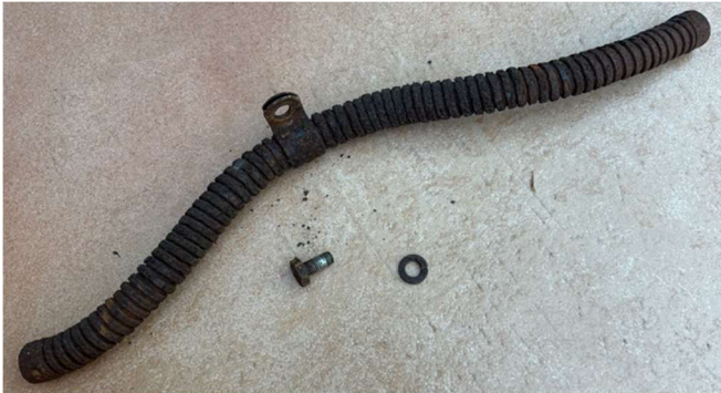
Original 6v battery link cable armoured protection casing
