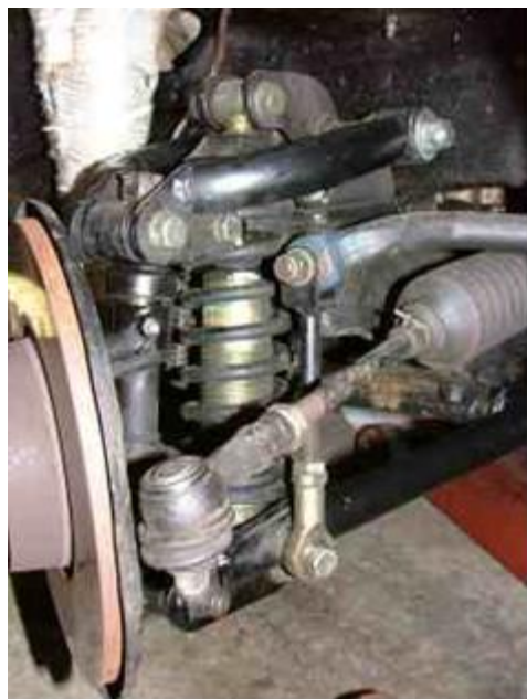
Front suspension with the coilover damper conversion (Photo: Geoff King)
