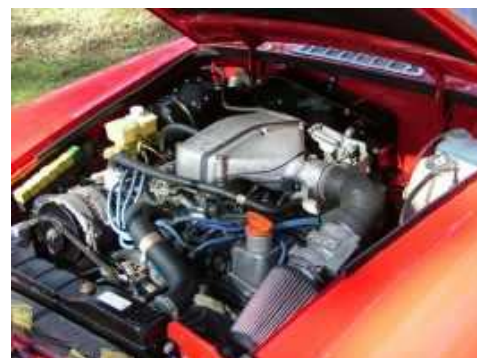
Engine bay is very neat with the injected V8 power unit. (Photo: Geoff King)
