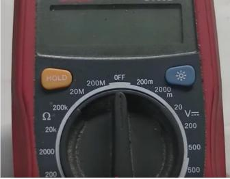
Using a digital multimeter to start the test, earth the condenser on its body to discharge it. Then set the meter to 20M in the Ohms  $\Omega$  section of the meter. Connect the probes to the body and tail - they are not polar sensitive. If it is good, the meter reading will rise up then stop at 1.
