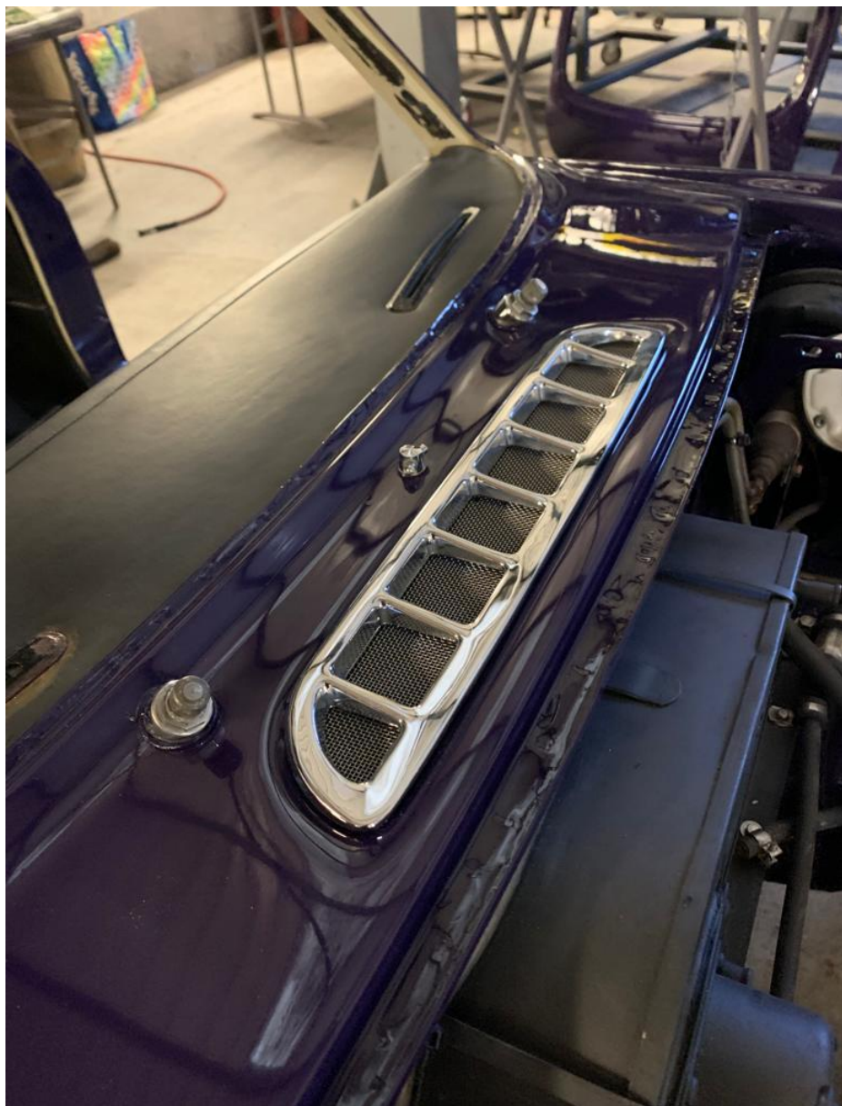
Air intake in front of the windscreen with an aftermarket mesh which keeps leaves out so they don't collect at the bottom of the air chamber with road dust.
