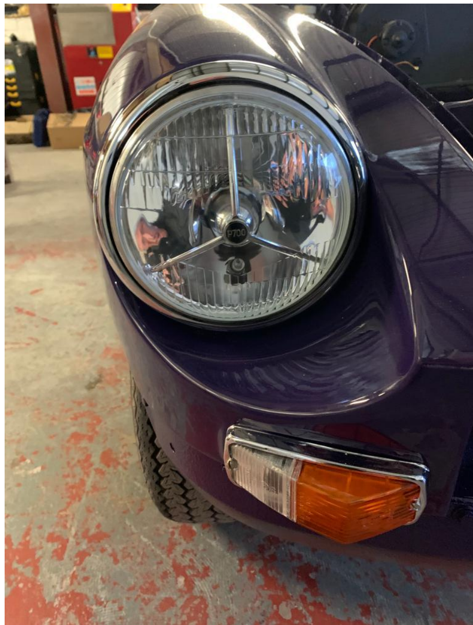
Upgraded front light & side light units fitted – the old sealed beams provide as much head lighting as candles! An upgrade well worth making.
