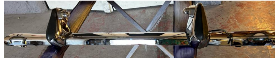
Rechromed rear bumper with the numberplate illuminators on the overriders. The work was carried out by a rechroming specialist in the West Midlands.
