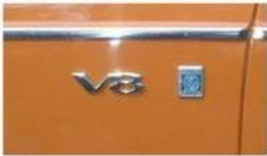
Location details for positioning the badges on the nearside front wing Note – no badges were fixed to the offside wing as it is so often seen with cars that have been refurbished at some stage. The V8 badge for the wing is flat.
