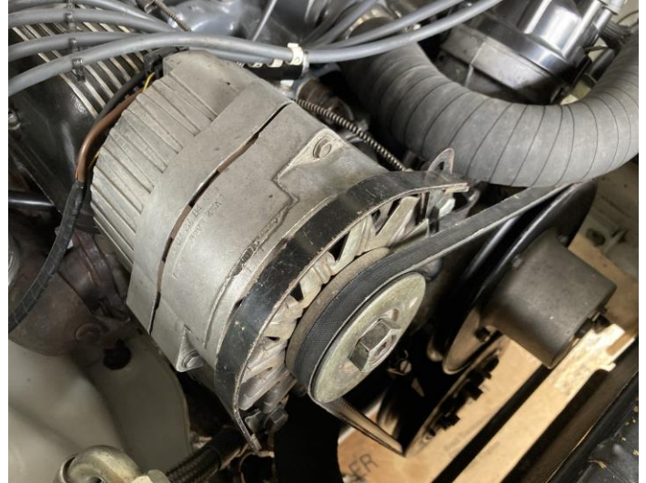
Fan guard fitted to a standard alternator on an MGBGT V8
