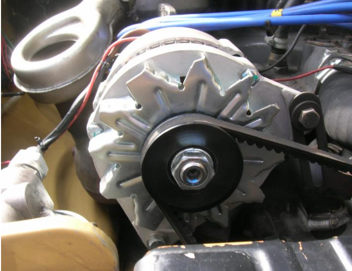
Bold fan blades on a 75amp replacement alternator
