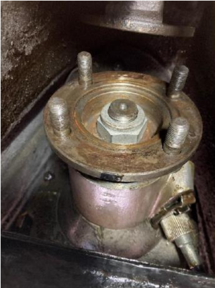
Figure 3 - Mark the relative position of nut and shaft with a centre punch to aid reassembly
