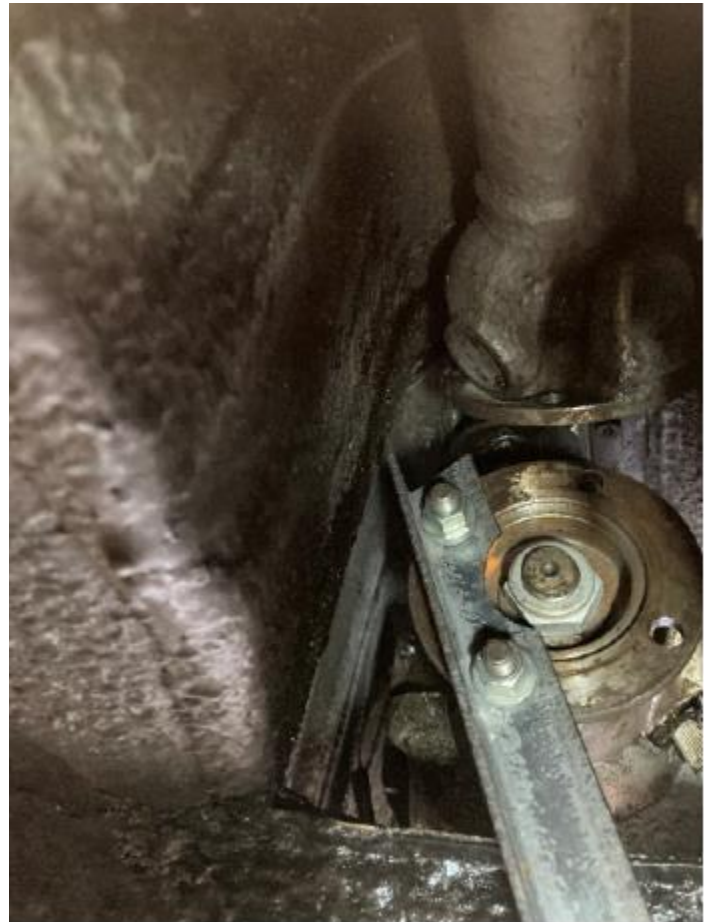
Figure 4 - Attach the restraining tool to the gearbox flange using two of the original bolts, spacers/washers and free running 3/8" UNF nuts
