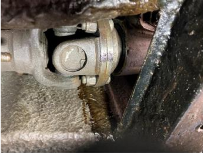
Figure 2 - Paint alignment marks on the gearbox and propshaft flanges to ensure reassembly in their original position
