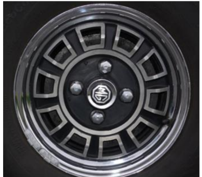
Original 14" Dunlop composite V8 wheel - chrome steel rim & alloy centre
