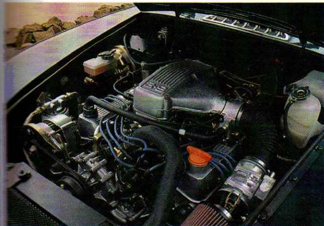
Land Rover's 3.9 V8 gives 187bhp, 231 lb ft torque
