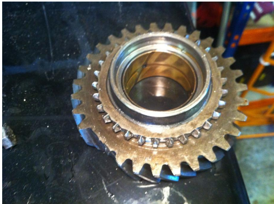
A few teeth missing from first gear - the probable result of V8 torque and too many wheels spins from stationary
