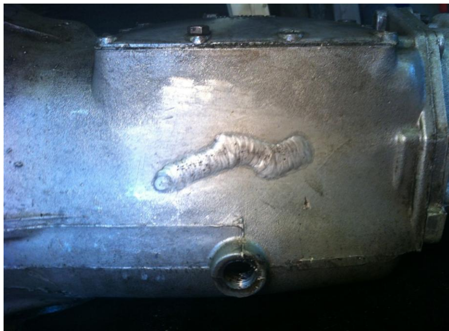
External view of the welded crack in the gearbox casing
