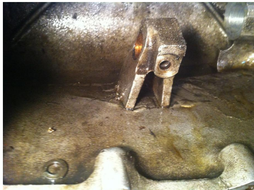
Internal view of the casing - the repair to the reverse shaft bracket is clearly visible as are weld fillets on the left hand side reattaching the bracket to the casing
