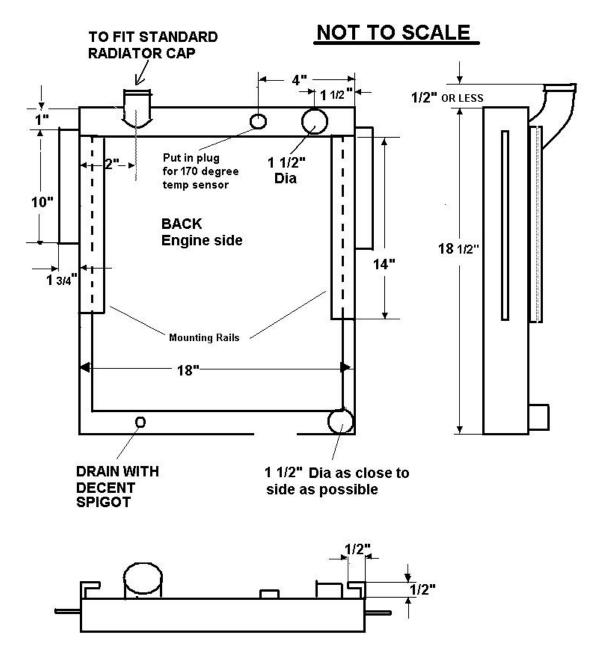
The idea with the 'mounting rails' is to make small angle aluminium bars from 3/8ths or such that can be bolted to them. Thus one could position an electric fan wherever it was wanted by drilling appropriate holes in rails and cross bars. These bars I can make myself but if you want to include two with the price......
