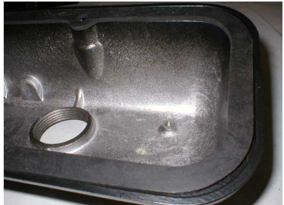
Factory MGBGT V8 rocker cover with a flat cork gasket fitted.
