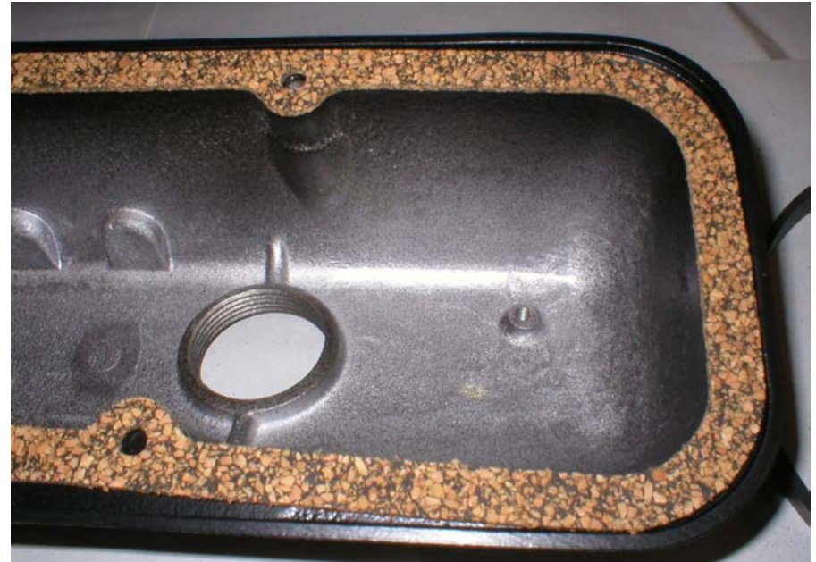
Factory MGBGT V8 rocker cover with a flat cork gasket fitted.
