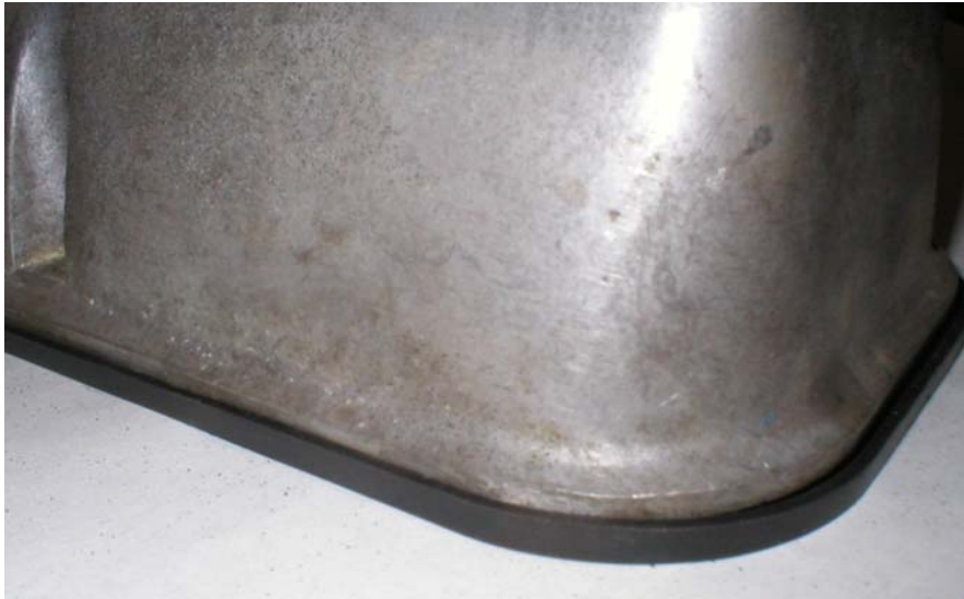
Outer view of an RV8 & SD1 rocker cover with the rubber gasket fitted
