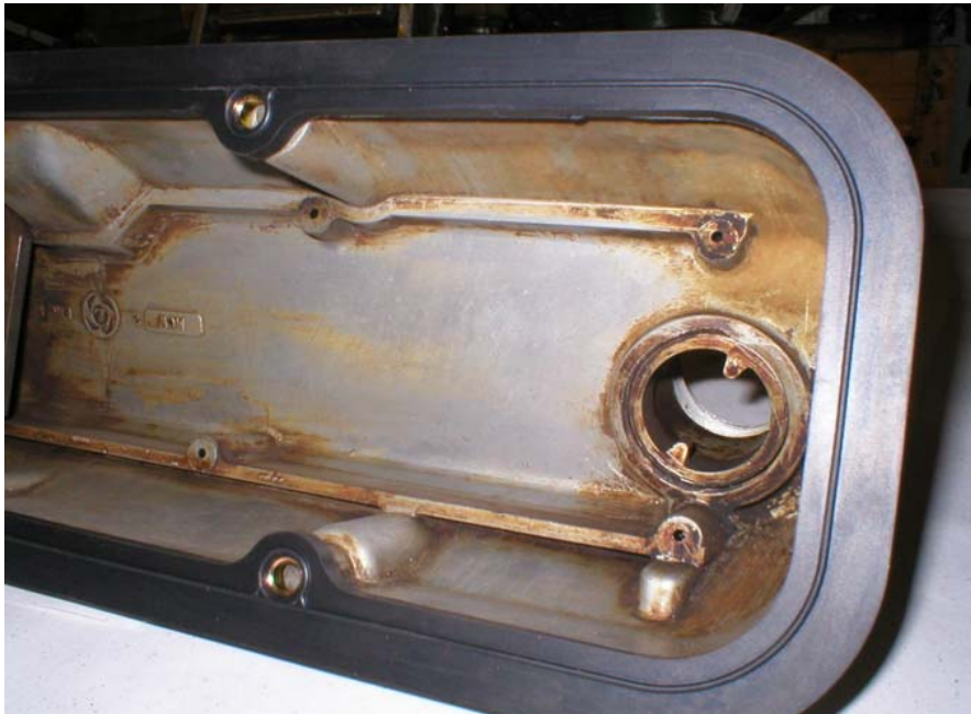
Underside of an RV8 & SD1 rocker cover with the rubber gasket fitted.
