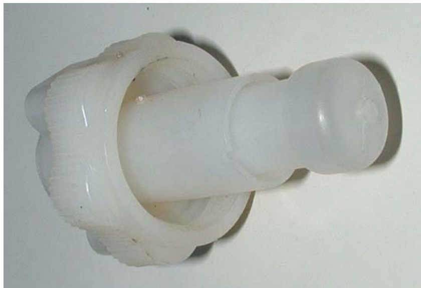
The float mechanism which fits in the brake master cylinder
