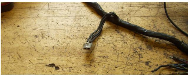
The wiring loom of my MGBGTV8 was not in bad condition, but they always have a few small problems. This one had a broken connector to one of the cooling fans - see photo above (Wiring 3).
