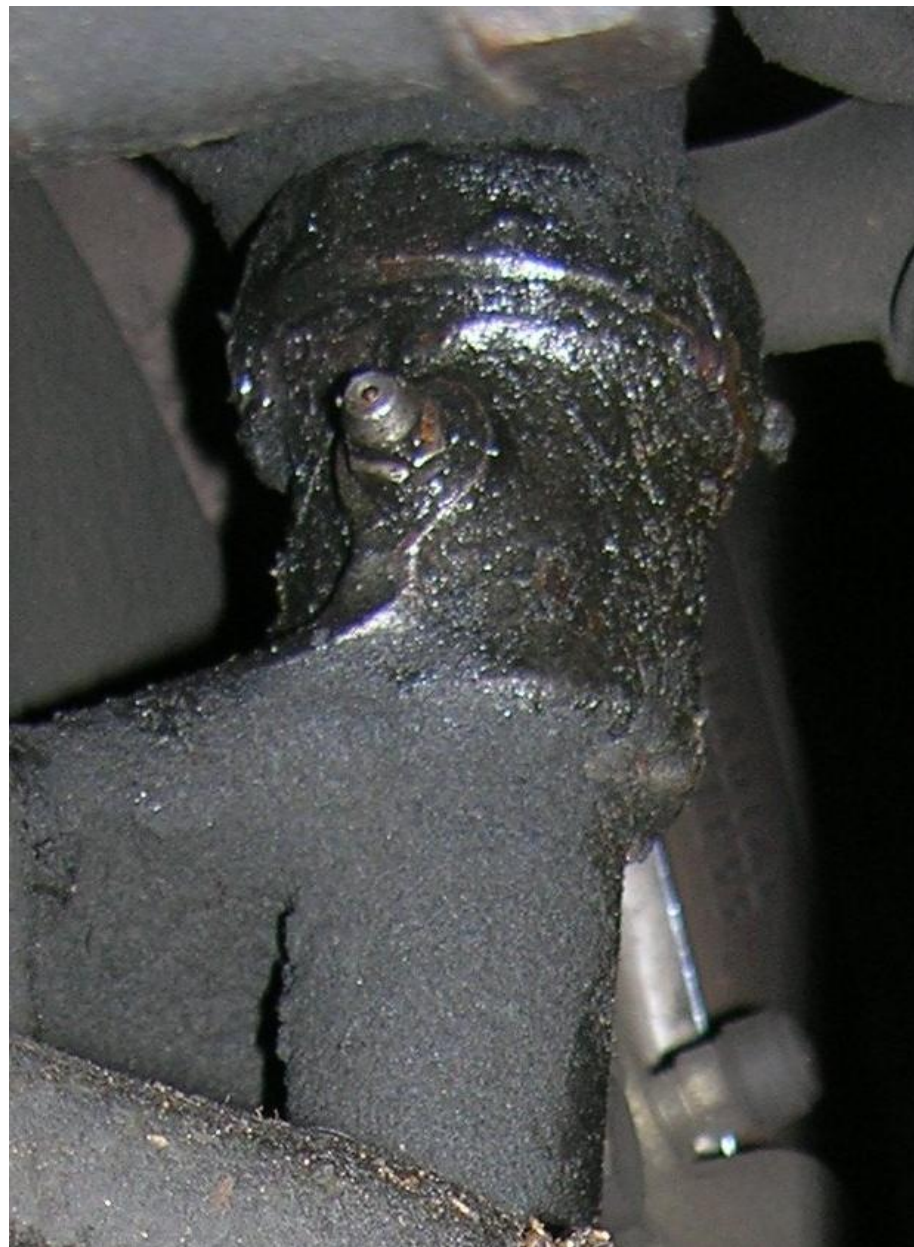
Four good pumps with the grease gun until clean grease emerges.
