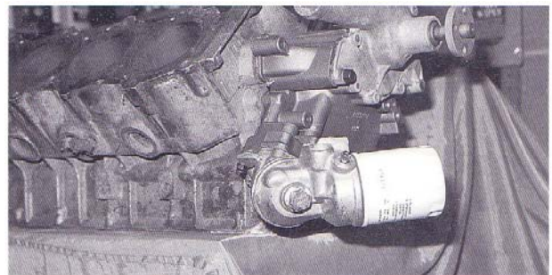
2-5-2-2 A rotatable oil-filter mount shown on a Buick V6 oil pump base.
