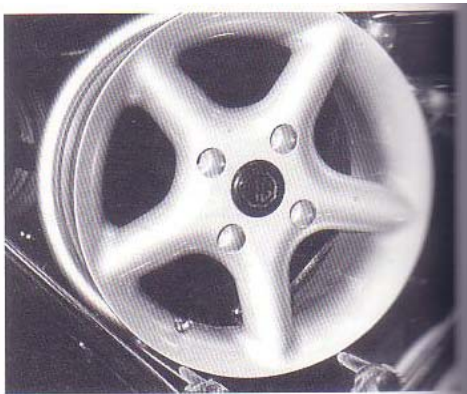
6-8 This is a 14 inch x 6J alloy wheel called Stealth. It is made by TSW but marketed by the MGOC – very smart too.
