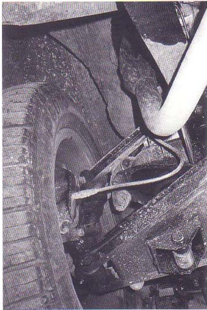
7-2-3 This front suspension improvement uses coil-over shock absorbers. The photograph shows the new spring pan and lower mounting method for this type of front suspension. You should also note the route of the RV8 exhaust system.
