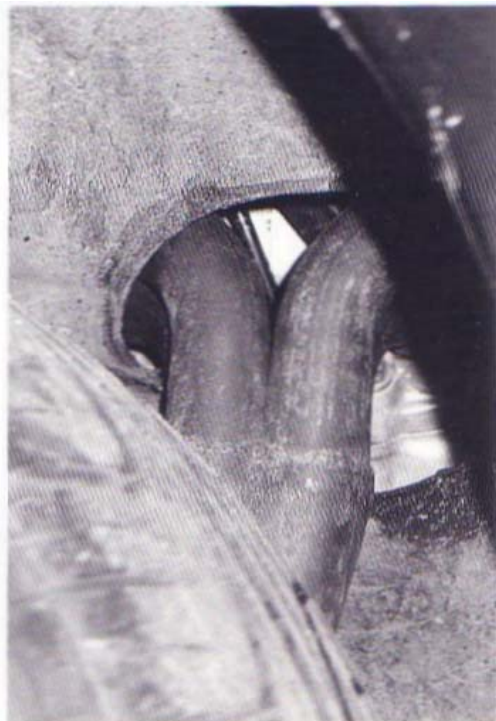
5-1-2 This photograph shows that the inner wing has been strengthened, in this case by turning down a lip. Most inner wing strengthening for RV8s is achieved by welding a "ring" of steel around the aperture.
