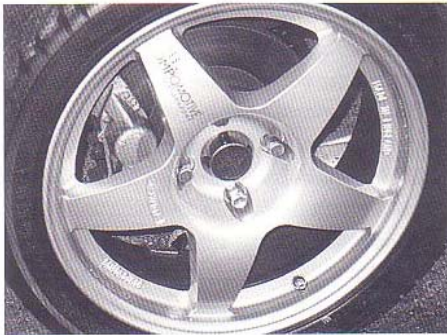
6-6 These superb Compomotive wheels have 7 inch rims and are running 205x50x16 inch tyres. These show off the brake calipers very well indeed (in this case, SD1 Vitesse), which are considerably wider than the Princess caliper shown in the preceding shot.
