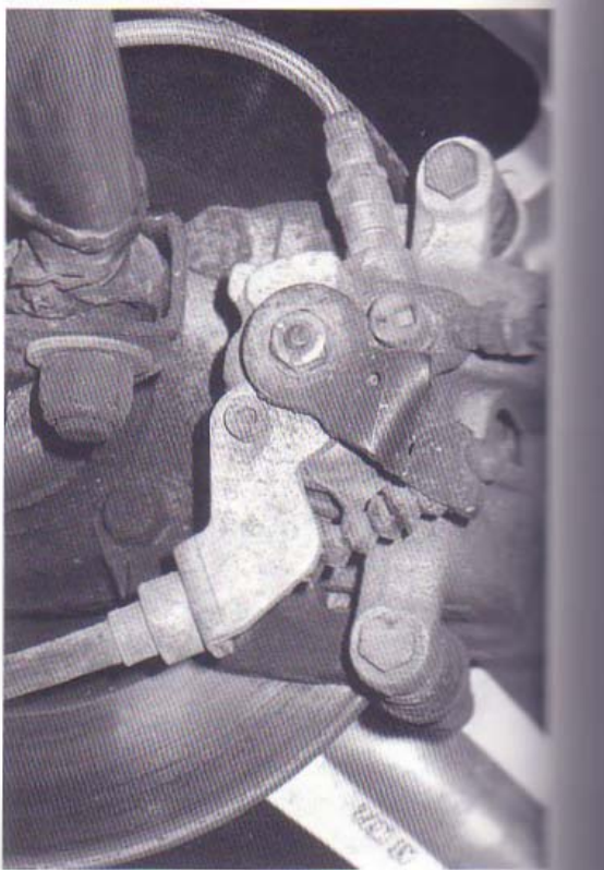
10-3-3 This is an MGB rear axle/disc brake combination. The mounting bracket bolts to the inside of the rear axle flange. An interesting bonus is the view of the rose ball joint on the end of this axle locating Panhard rod (top left of the picture).
