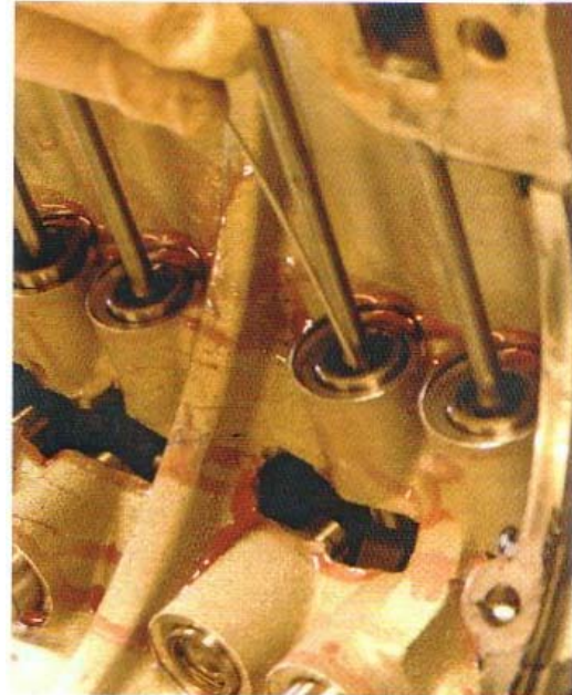
2-7-15 Using 0.060in diameter wire for the high tolerance cam-follower pre-load check.
