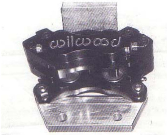
10-2-10 Wilwood's Dynalite caliper with adapter bracket pre-fitted.
