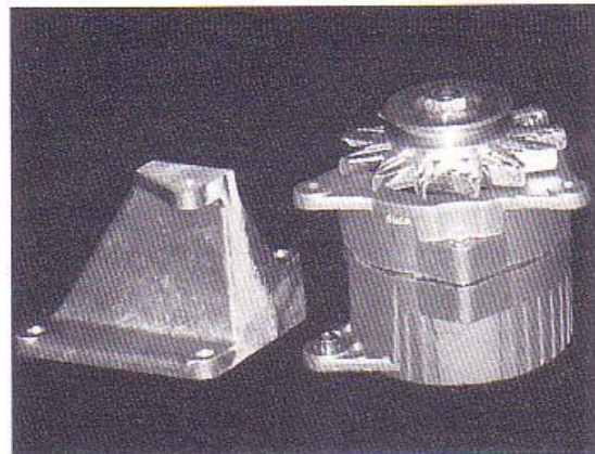
13-1-4 The traditional 45 amp MGB GT V8 alternator and excellent reproduction V8 mounting bracket available from Clive Wheatley,
