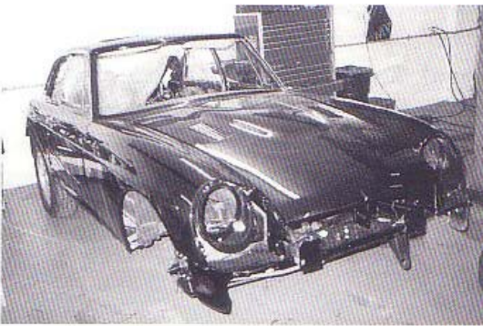
9-4-4 The same shell, of course, from another angle. It is difficult to appreciate, even from this angle, but the RV8 panels have the practical benefit of allowing wider track and/or tyres.
