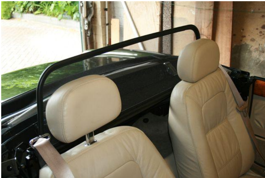
New German wind stop improves comfort for both driver and passenger with the hood down
