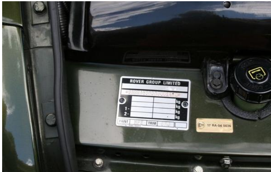
VIN plate attached to the slam panel with the hydraulic filler and cap alongside for the electro-hydraulic power assisted steering system installed as a retrofit.
