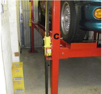
Alan Aldous says "I have a car lift in the garage in case of a flood (it's also has been known to be used for work on car!) and you can see the very basic 'farm jack' at each corner that requires three 'pumps' to lift the 3 inches, this allows the second safety bolt to be fitted before the first is removed to lift a further 3 inches etc. I take it a corner at a time when I have used it. It's a HAMER car lift."
