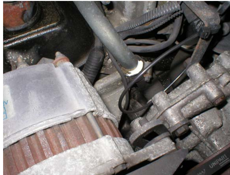
Above: showing the front cover to heater rail hose in place. The heater rail runs along the top of the engine back to the heater and is fixed by a bracket across the engine
