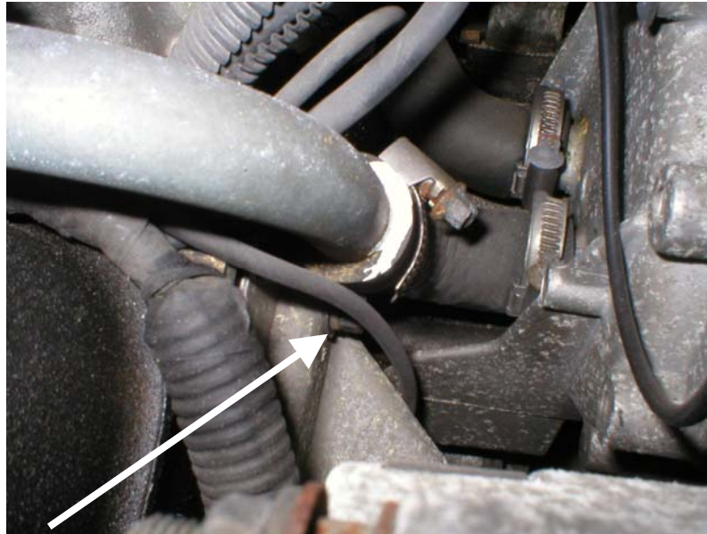
Heater rail pipe showing the alternator bolt that can get pushed into the rubber hose below – it's just in view bottom left of photo above
