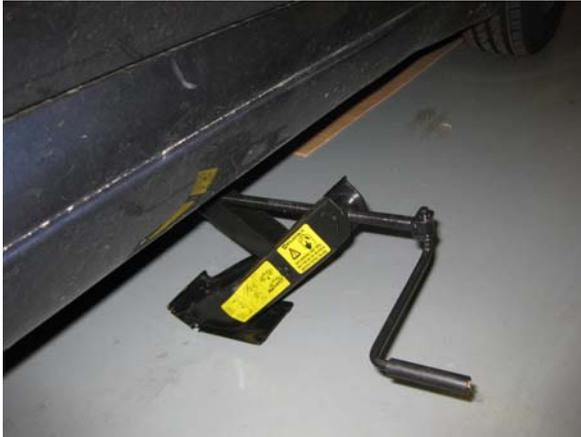
The original jack is of the half scissor (aka a Y or boomerang) design and is raised or lowered by a handle which operates a screw mechanism. The jack, including the screw mechanism, should be sprayed satin black.
