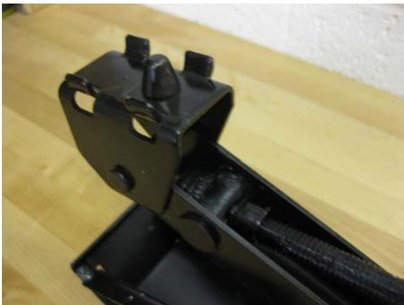
There's a locating peg which fits in the car's jacking point. The jack can be readily identified by the two gummed yellow paper labels which should be attached thereto. The larger label shows three pictures:
