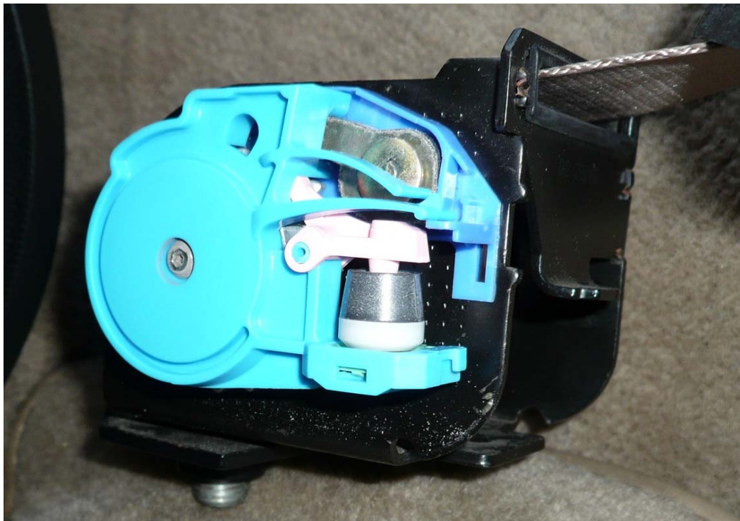
Mechanism exposed. The metallic item, top right in the blue area, is the main inertia catch. The grey/pink cup bottom right in the blue area is the "tilt sensing" device and the pink lever above it is the catch that rests in the cup when the reel is unlocked. (Photo: Erik Persson)
