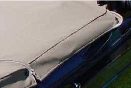
Stud fixing on the generous overlap section over door capping and another behind the door on the tonneau section over the folded hood
