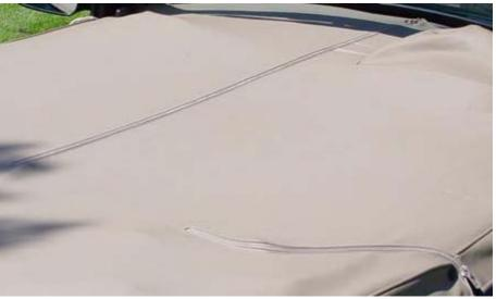
Stud fixing on the top of the panel above the dashboard, the full length zip, side zips behind seats to facilitate folding the tonneau sections behind the seats. Note the generous overlap section over the door capping with the stud fixing near the wing mirror
