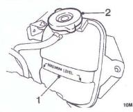
Visually check that coolant is not below the level marked on expansion tank. If level is appreciably low, suspect leakage or overheating.
