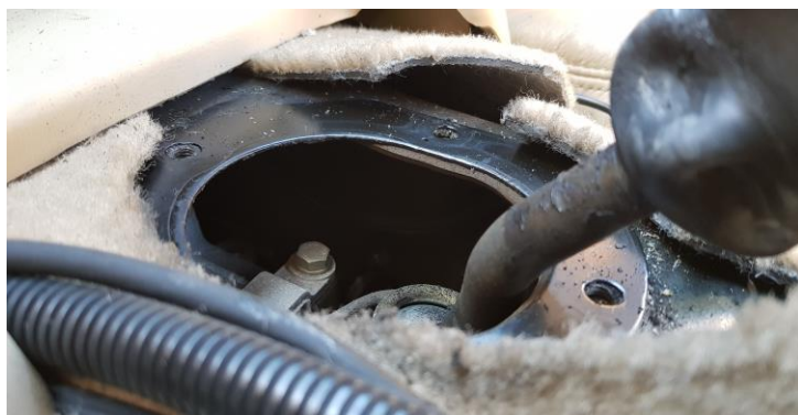
RV8 – contact between the gear lever and the edge of the opening
