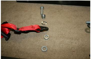
Now fit the rectangular plate in the kit to the mounting surface of the belt reel as below with a piece of duct tape. You might be able to fix it without doing this, but it prevents the plate from rotating out of place as you tighten the bolt. The dimples in the plate should engage with back of the reel, this provides reinforcement for the
