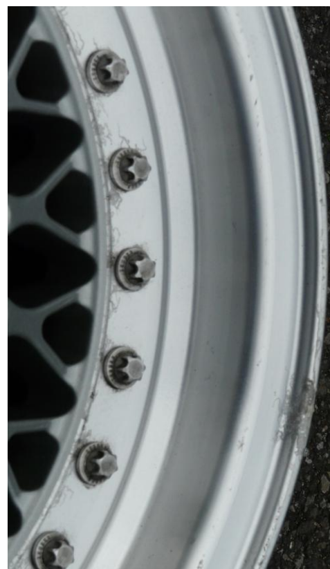
Top left: emphasises the excellent finish achieved on the refurbished wheel centre and cap. Above: before refurbishment showing lacquer lifting. (Photos: Al Barnett)
