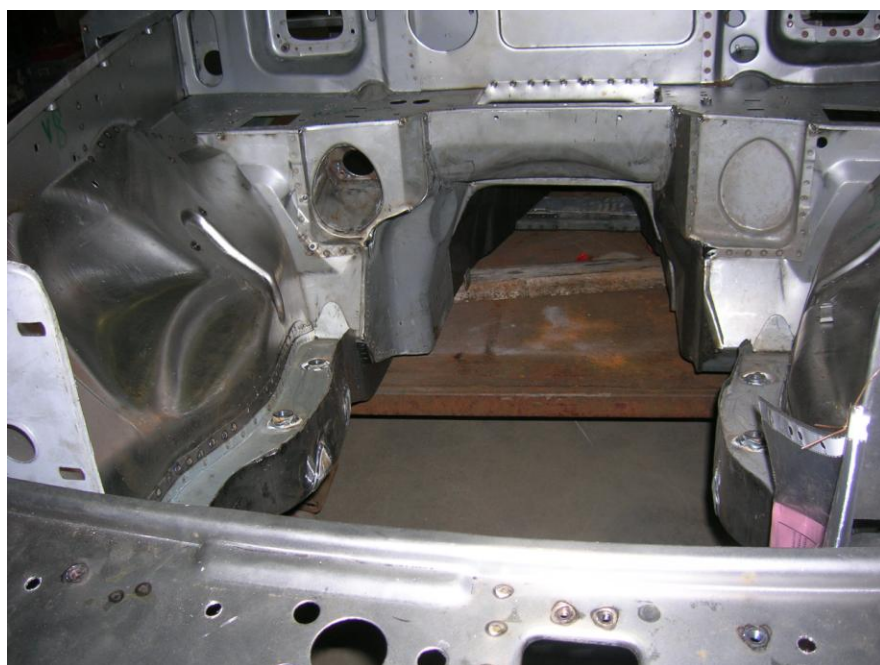
Bulkhead of a RHD MGB Roadster opened up for a Rover V8 engine and gearbox with the LHD steering column opening closed.
