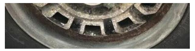
Above is an example of a Dunlop composite wheel on an MGBGTV8 "barn find" which was in a seriously corroded condition. The chromed steel rim is looking rough and the section of the rim near the alloy centre is particularly corroded.
