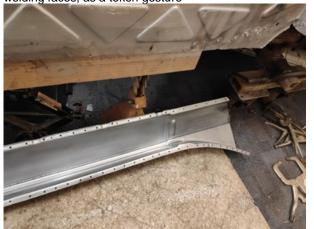
With a good grind and wire brush applied a coat of epoxy sealer to all the inner sections and rear wing internals and trial fitted the rear wing and door. Much better.
