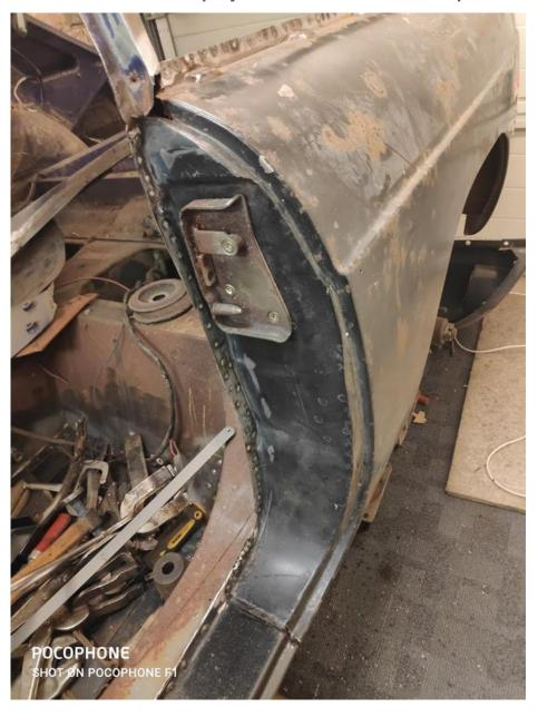
The rear heelboard extension piece was rusty and cut out. Again a where not being welded a coat of epoxy sealer and then on the weld thru edges a coat or zinc weld primer. Also a small section of the spring hanger needed replacing, hadn't rusted thru yet but now it was easier now than later on. Got carried away with the hole punch here but this was almost the same amount that the OE piece had in it, just means a load of grinding coming up.
