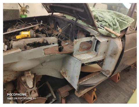
Footwell side in and a bit of wing gutter replaced. Didn't get a photo of the inner wing turret before I got the front wing on for a trail but I can update this later.
