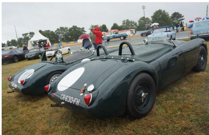
MGA Le Mans Replica of Christian Lissot with a 2 litre engine, cross flow head, and two 45 twin Weber carburettors.
