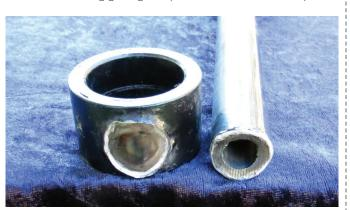
Weld penetration and metal added by the welding were both minimal on the original lateral links fitted to Malcolm's 260.
