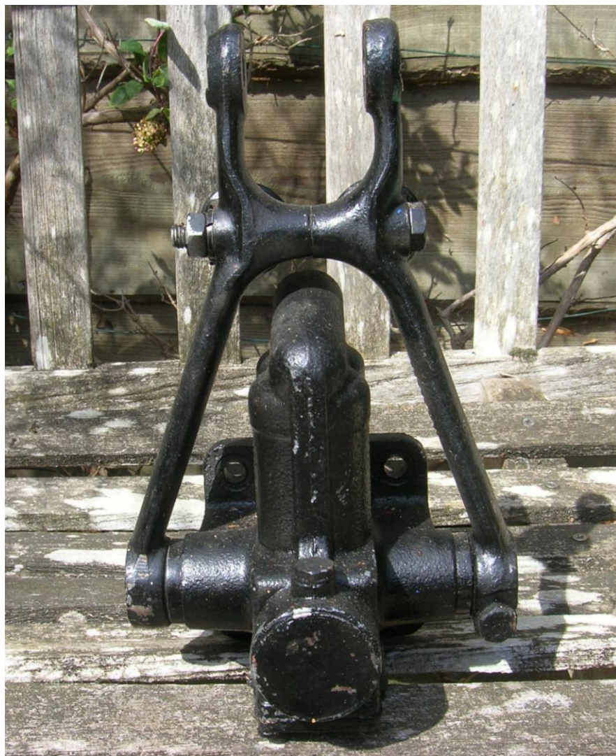
Pair of front MGB dampers, part number GSA119 in good condition.
