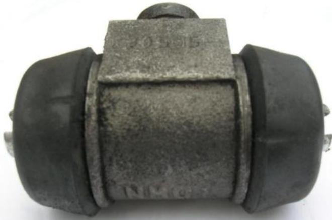
Rear brake wheel cylinder assembly with seals at each end
