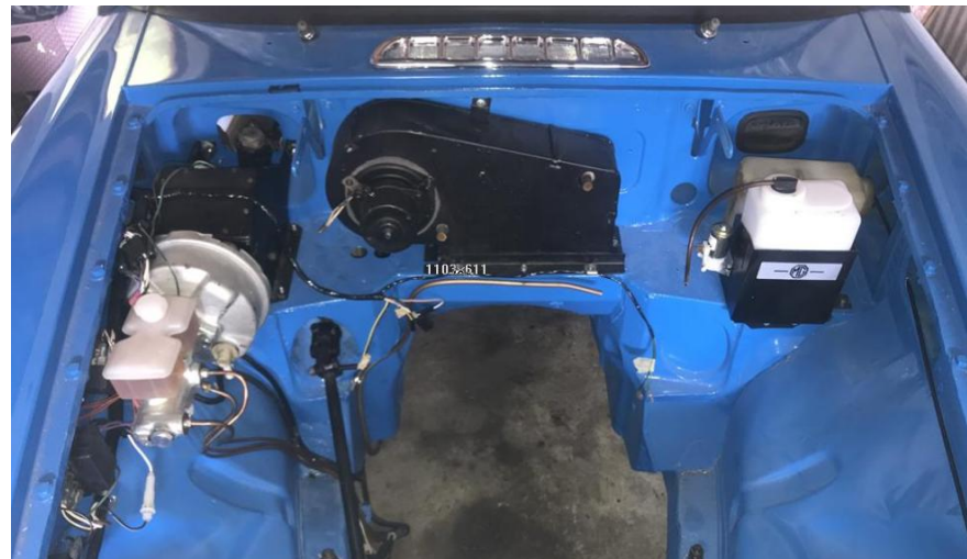
MGB Roadster engine bay ready for the V8 engine to be installed
