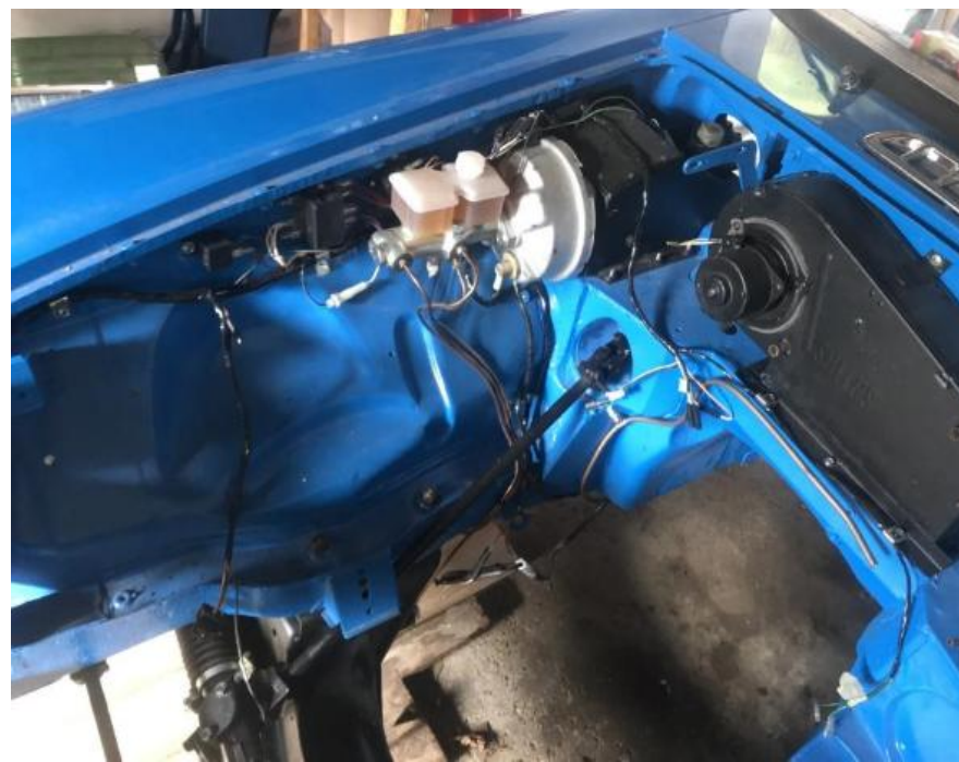
New servo and new master cylinder were part of the upgrade
