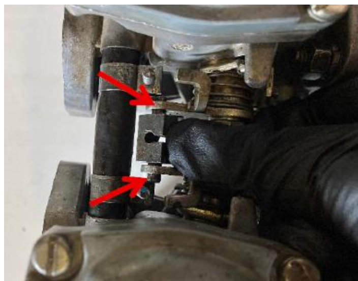
Figure 3 - foul between ears of the hose clip and choke trunnion (from below)
