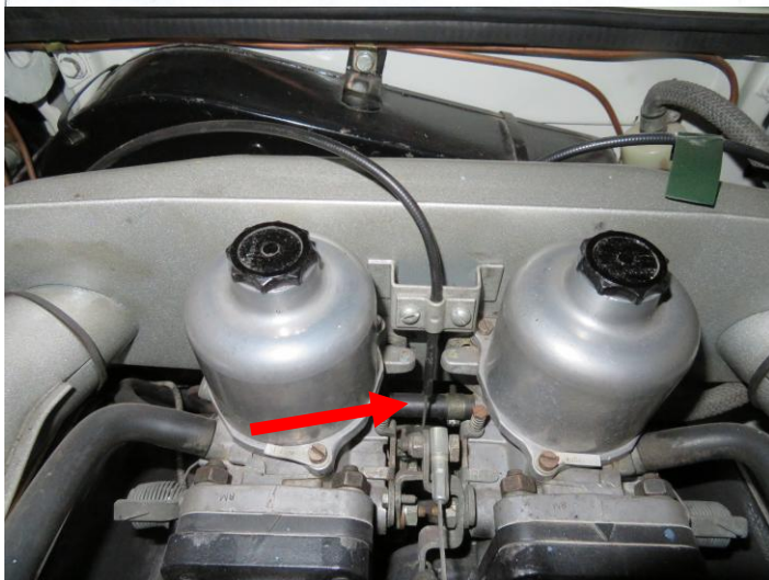
Figure 1 – leaking hose between the carburetors
