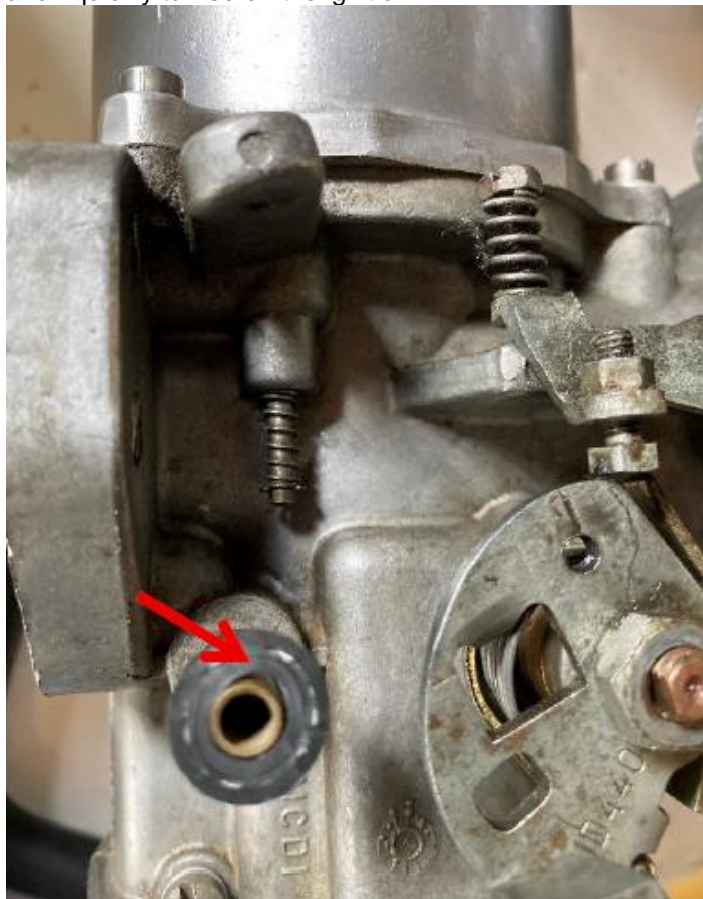
Figure 4 - ovality remained with a clear gap between hose and pipe
