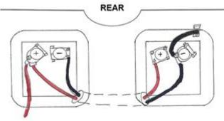
There is a protective sleeve through the tunnel over the propshaft. A larger copy of the illustrated guide to installing the twin 12v battery wiring kit is available online. See link to the wiring layout
