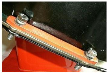
Engine steel sump upgrade kit - the steel plate is 5/8" x 11/64" with 18 bolt holes at 25/64" with a plated finish on the support plate.
