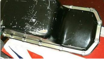
Classeparts' new steel support plate has been produced to snuggle fit between the sidewall of the sump pan & the short 90 Deg outer flange
