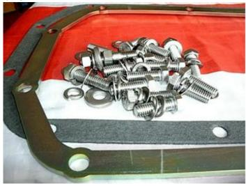
The kit comprises a sump gasket, mild steel plate with a surface finish zinc and colour passivate and a set of stainless steel fittings comprising nuts, bolts (longer than the originals to account for the thickness of the plate), studs and washers. The steel support plate is 5/8" x 11/64" with 18 bolt holes at 25/64" with a plated finish.
